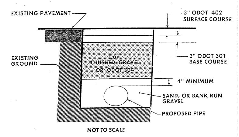
MINIMUM TRENCH WIDTH WIDTH SHALL BE I.D./PIPE PLUS 2'0"
